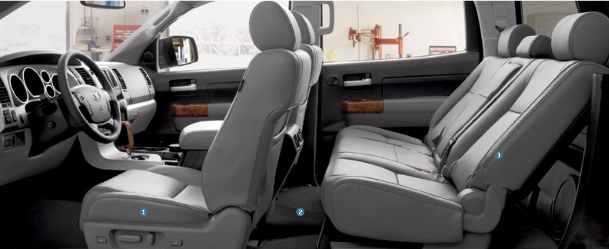
[1] POWER THIGH SUPPORT On available models, the Power Thigh Support features a driver's seat with a seat cushion extension that provides additional support.
