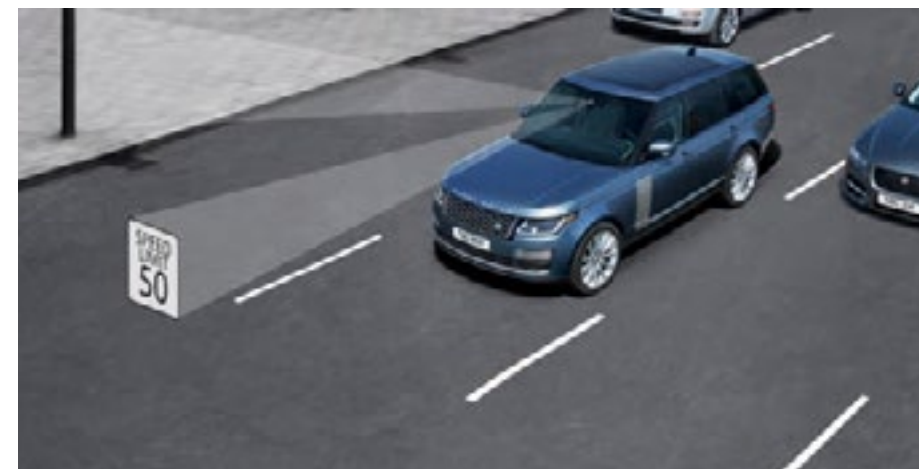
Traffic Sign Recognition with Adaptive Speed Limiter
