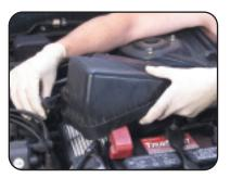
**△WARNING:** Severe and costly damage may result if airflow meter screws are removed
