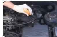
RELEASE THE RETAINING CLIPS -Release each retaining clip around the rim of the air filter cover for both carbureted and fuel-injected systems.
