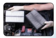
**NOTE**: If the element is just moderately dusty, it may be cleaned by blowing compressed air from the inside outward or from the downside upward. NEVER wash or oil the element.
