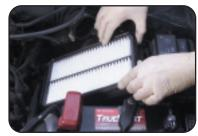
PLACE THE AIR FILTER COVER IN POSITION -Align the arrow on the cover with the arrow on the air filter case (if so marked).
