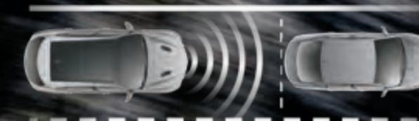
**Adaptive Cruise Control with Stop & Go (ACC Stop)<sup>10</sup>** This available system helps drivers maintain a safe distance from the vehicle ahead and, under certain traffic conditions, the system can bring the Stelvio to a full stop without driver intervention.
