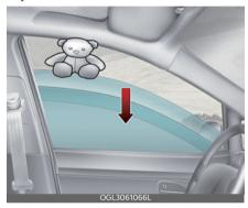
If the window detects the resistance while the power window switch is pulled up continuously, the window will stop upward movement then lower approximately 1 inch (2.5 cm).
