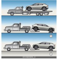
Proper lifting and towing procedures are necessary to prevent damage to the vehicle. The use of wheel dollies (1) or flatbed is recommended.
