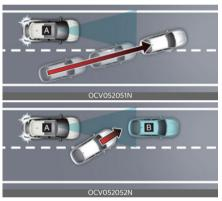
[A]: Your vehicle, [B]: Front vehicle If a vehicle cuts in front of your vehicle, Leading Departure Alert may not operate properly.
