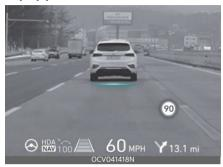
The Head-Up Display projects the instrument cluster and navigation information onto the windshield.
