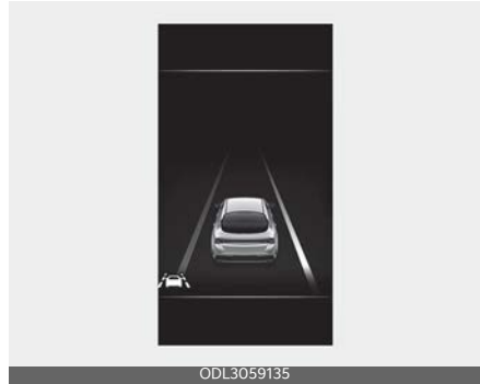
Lane departure warning (right)
