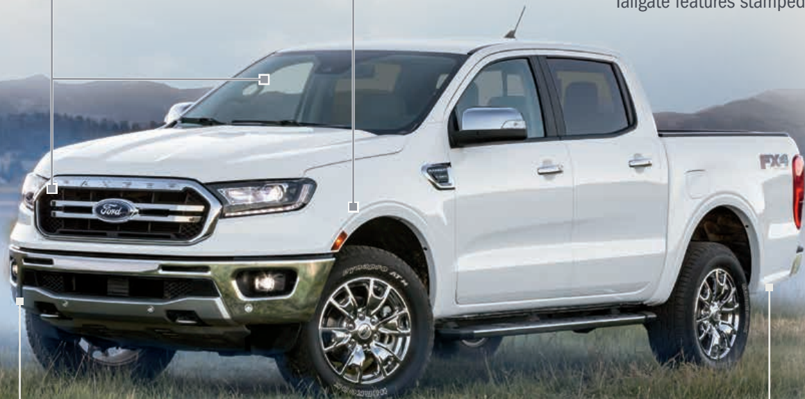
Short front and rear overhangs as well as high ground clearance for off-road capability.
