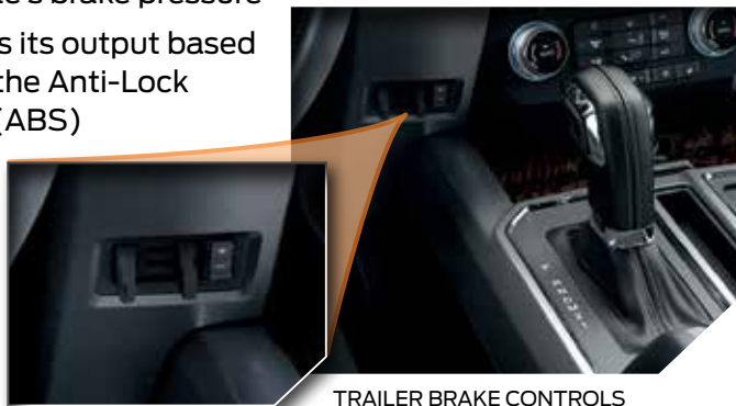
TRAILER BRAKE CONTROLS
