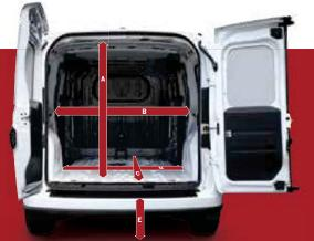
A. CARGO AREA HEIGHT 51.8 INCHES B. CARGO AREA WIDTH 60.4 INCHES C. CARGO AREA LENGTH 87.2 INCHES BEST-IN-CLASS[10] CARGO CAPACITY 131.7 CURIC FT D. BEST-IN-CLASS<sup>(10)</sup> CARGO WIDTH BETWEEN WHEEL WELLS 48.4 INCHES E. REAR STEP-IN HEIGHT 21.5 INCHES BEST-IN-CLASS[10] PAYLOAD (CARGO VAN MODELS) 1.883 POUNDS
