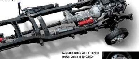
WE LOOKED AT THE DESIGN FROM THE UPFITTER'S POINT OF VIEW, and it's why we put a premium on maintaining rigid standards. This heavy-duty flat frame features 34-inch rails, with all components outside of the main upfit areas. That best-in-class<sup>[9]</sup> rear frame strength of 50,000 psi on Ram 4500/5500 clinches the deal.
