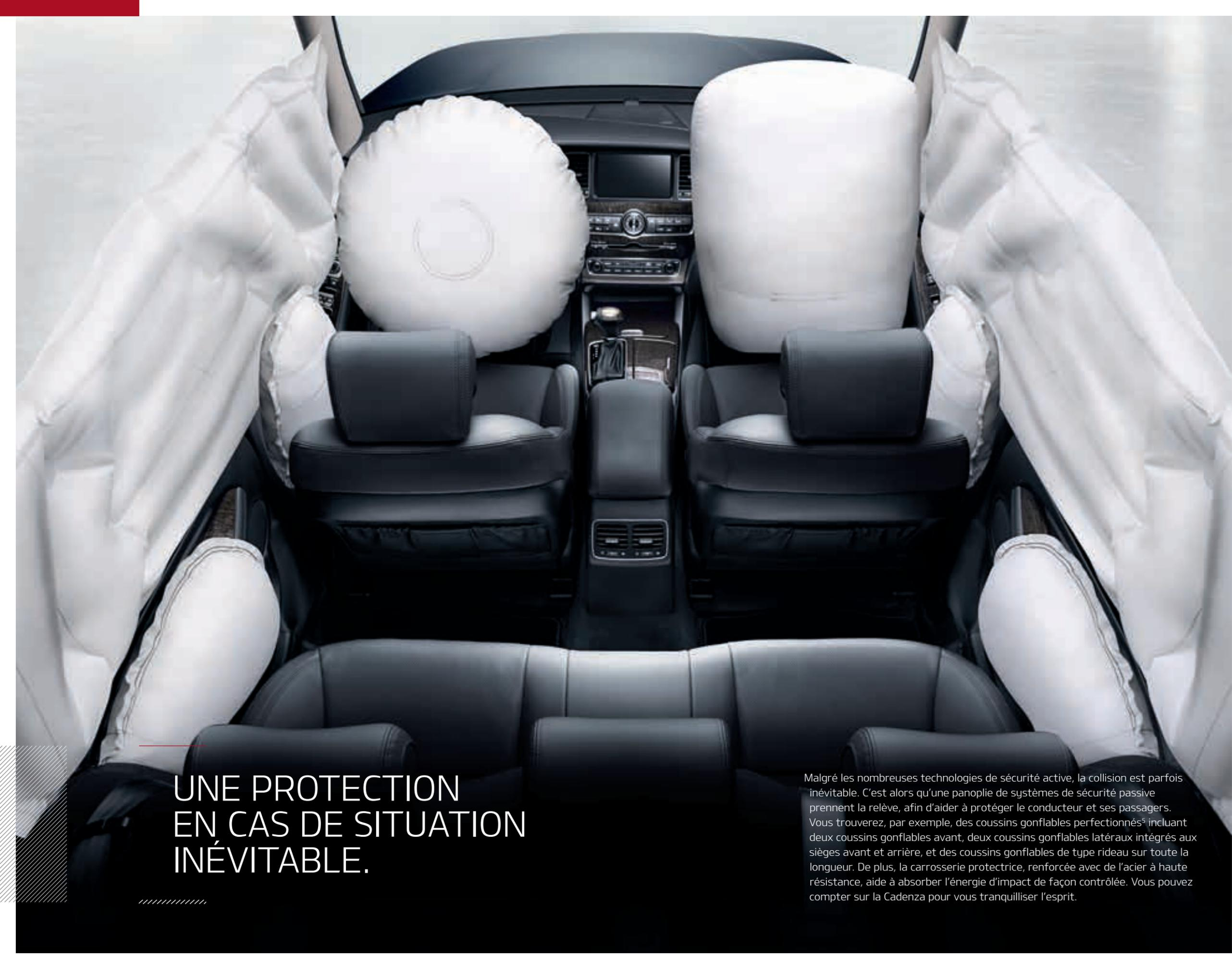
A black and white photograph showing the interior of a car from a rear passenger perspective. The front seats are black leather. Two large, white, circular airbags are deployed from the front seats. Two white, side-impact airbags are deployed from the outer edges of the front seats. A white, curtain-style airbag is deployed from the ceiling on both sides. The center console and dashboard are visible in the background.
