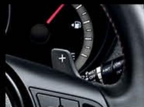
**PADDLE SHIFTERS.** Forte SX models equipped with the available 6-speed automatic transmission feature paddle shifters that allow you to change gears without taking your hands off the wheel.
