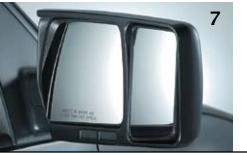
7. Removable Trailer Tow Mirrors: Ideal for occasional towing, they slide easily over existing mirrors to enhance rear vision when pulling
