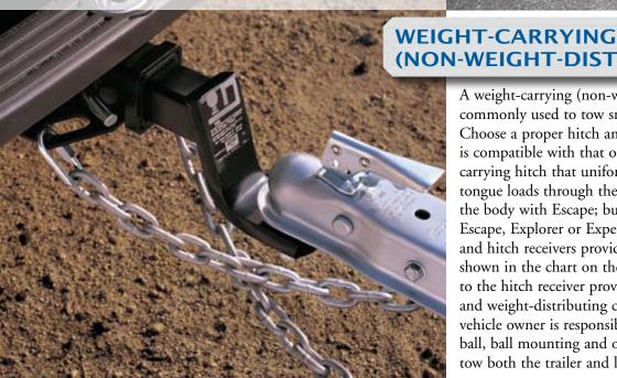
(NON-WEIGHT-DISTRIBUTING) HITCH A weight-carrying (non-weight-distributing hitch) is commonly used to tow small and medium-sized trailers.
