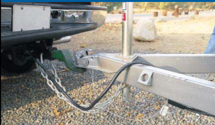
Trailer wiring harness and frame-mounted hitch receiver (shown with aftermarket hitch equipment).
