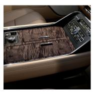
Wireless charging; standard Wi-Fi: The all-new Navigator is the first Lincoln to offer wireless charging. The wireless charger is a flat pad rubber surface in the media bin located next to the dual USB charge/SYNC data ports. When charging a phone equipped with wireless charge capability, a popup at the top of the screen indicates that the wireless charger is active. Standard Wi-Fi allows up to 10 mobile devices to be connected. and there are power outlets and USB ports for each row.
