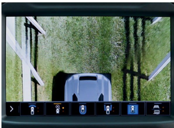
Front Top-Down View Provides a top-down view of the hood, bumper and front tires for tight manoeuvres in parking lots or along curbs.
