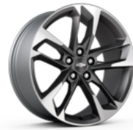
20" x 8.5" front and rear blade-design aluminum (Q7F) Available on 2LT and 3LT 3
