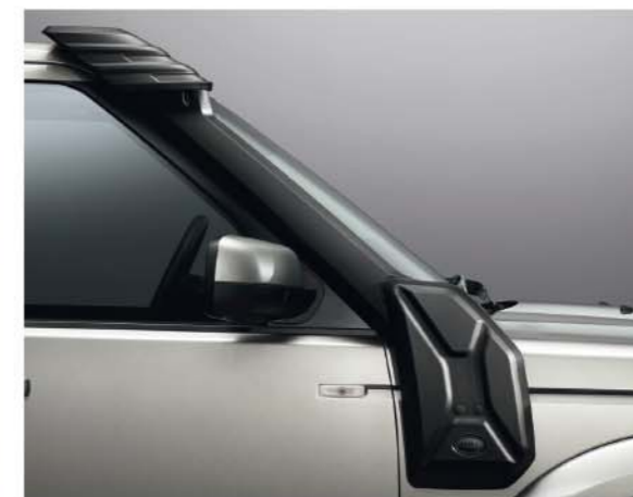
Raised Air Intake Not compatible with 5.0L V8 gasoline models. Additional parts are required for 3.0L TDV6 models. Please see your Land Rover retailer for more information. This accessory is not available for 2010 model year vehicles. For 2005-09 vehicles — ADL780010
