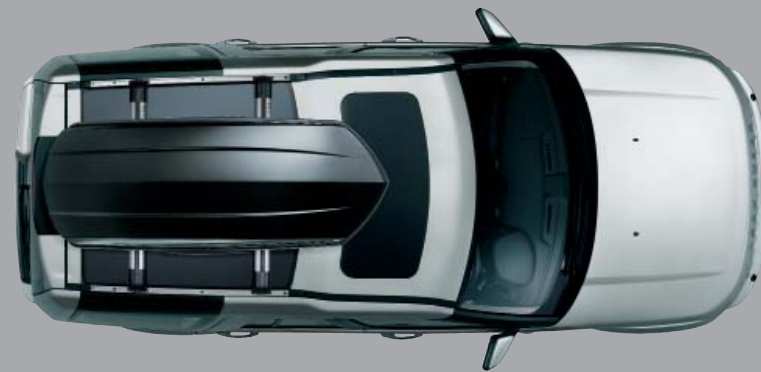
Sports Roof Box – Gloss Black Finish* Lockable for security. Can be mounted either way for curbside opening in any country. Internal retention system for skis or other long loads. External dimensions: 81" long x 33" wide x 13" high. Volume: 92 gallons. Load capacity: 165 lbs. VPLVR0061
