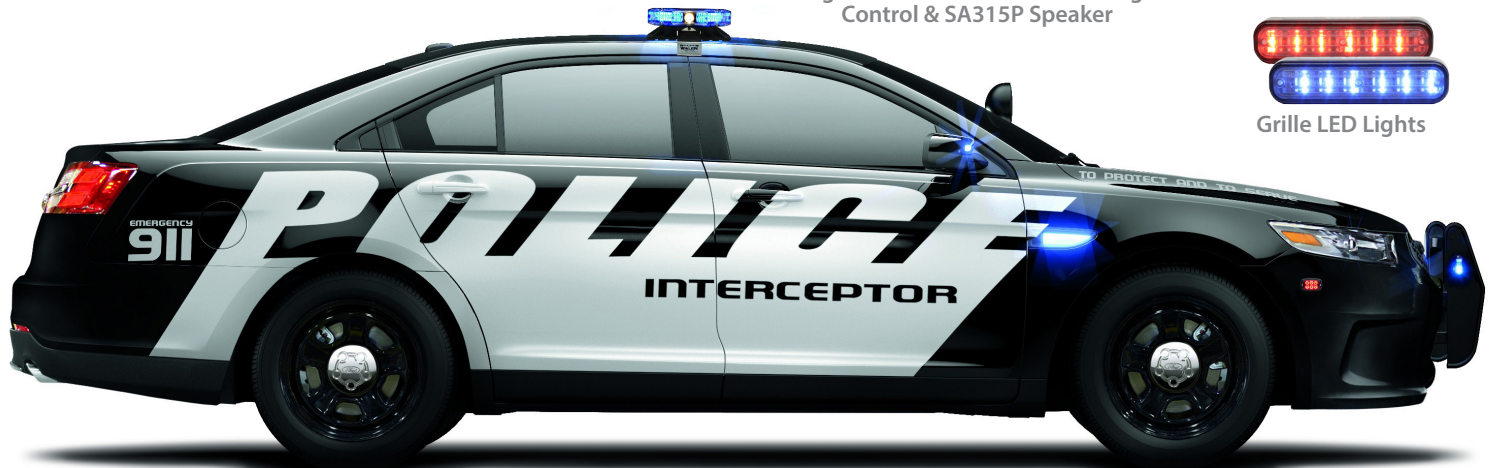
Single Unit Siren with 9-Switch Light Control & SA315P Speaker
