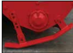
Tilling depth is controlled by adjustable skid shoes - to a maximum 8" depth.
