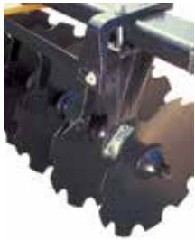
Standard Ductile cast rigid bearing hanger with regreasable flanged type ball bearing.
