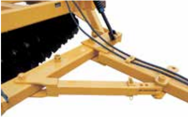
Telescopic tongue for easy adjustment of side draft
