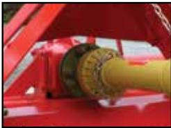
540 RPM Slipclutch drive line standard on Taylor-Way tillers.
