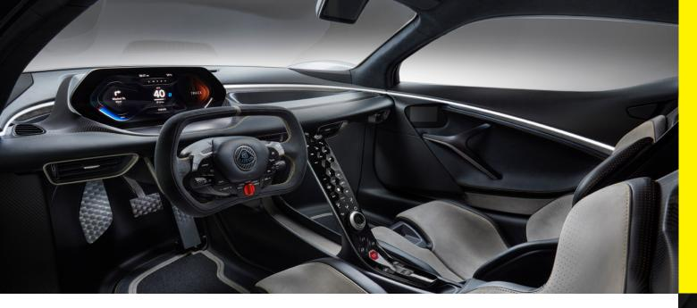
Ahead of the steering wheel is a state-of-theart digital display, providing the driver with key information such as mode, battery charge and remaining range. It is the car's only screen, putting all necessary information in one place. The screen displays essential functions only, with information appearing as required when the appropriate button is pushed, then fading when no longer needed.
