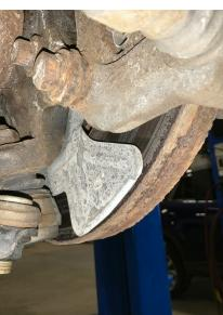
**Finding:** Pads at 0mm. Front brakes pulsing, pads heavily worn and rotors rotting. Calipers and slide pins OK at this time. Recommend replace front brake pads and rotors.
