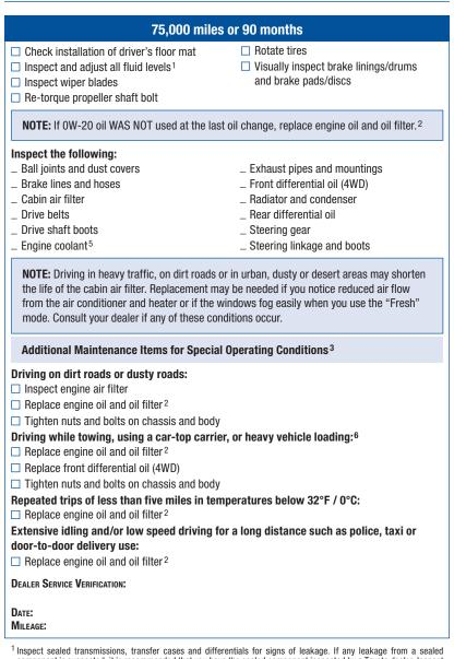
Inspect sealed transmissions, transfer cases and differentials for signs of leakage. If any leakage from a sealed component is suspected, it is recommended that you have the sealed component inspected by a Toyota dealer. Inspect power steering fluid (if equipped) and brake fluid level/condition. Inspect engine and inverter (if equipped) coolant level/condition/freezing point. Your dealer may recommend services (Dealer-Recommended Maintenance) based on inspection results.
