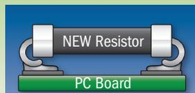
New, re-engineered resistors feature robust “shock-absorber” electrical leads.
