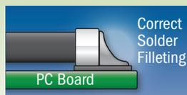
Correct solder filleting of re-engineered Genuine OE resistor leads ensure proper electrical contact and resist cracking.
