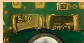
Hot-melt glue drizzled over resistors can lock in damaging heat.
