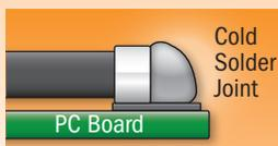
“Cold” solder joints may be present, resulting in poor electrical contact, cracking and component failure.
