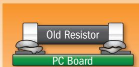
Reused resistors result in crack-prone electrical leads.
