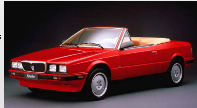
Years of production: 1982-1989 Numbers produced: 11919 Engine: 90° V6 twin turbo 18v, 2.0L, 180-223 hp
