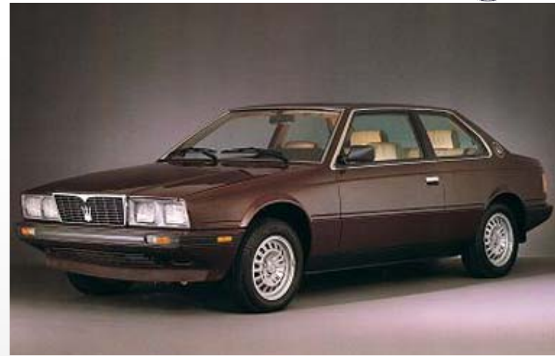
Years of production: 1982-1989 Numbers produced: 11919 Engine: 90° V6 twin turbo 18v, 2.0L, 180-223 hp
