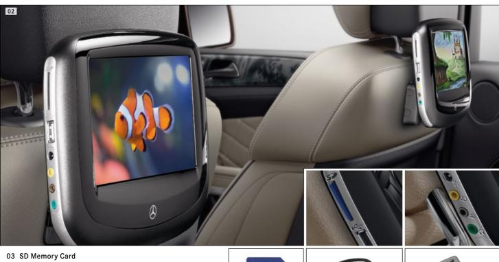
The COMAND system and Rear-Seat Entertainment System in your M-Class feature a slot for SD Memory Cards. Use the SD Memory Card as a convenient way to play music through the vehicle's loudspeakers while used with COMAND or view images on your Rear-Seat Entertainment System. Can also be used in other compatible devices such as digital cameras.
