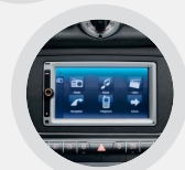
Audio system navigation/multimedia: the multimedia system has a 16.5 cm (6.5") touchscreen display, navigation with perspective map display and voice control, Bluetooth ® hands-free function for your telephone, AUX/USB port for your mobile music player, iPod ® interface that allows you to see your iPod ™ on the touchscreen, CD/DVD player, picture viewer and many other functions.
