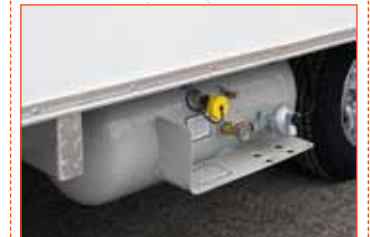
Underslung Propane Tank with Deckover Models
