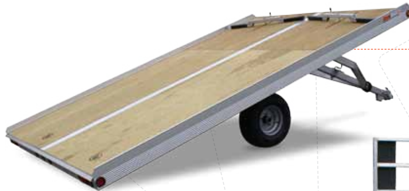
[22' DRIVE-ON/OFF] *Shown w/ Optional Deluxe Drive-On/Off Salt Shield and 15" Tire Upgrade
