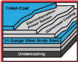
**A** Rugged 14 gauge two-sided A-40 galvanneal steel body shell with a six year warranty. Complete undercoating provides an additional layer of corrosion protection.
