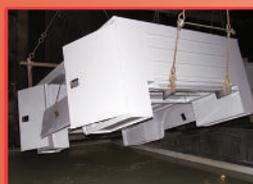
Rust shouldn't be a concern when you buy quality Knapheide we installed our state of the art, custom-designed electrodeposition an electroplating process, to give you a superior coat of primer methods. Complete immersion in our E-coat results in a prime Rust never sleeps, and neither does our E-coat protection so you
