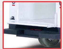
**M** Slam lock tailgate with one hand center release for convenience. Durable double panel construction has flat interior surface for work bench use.
