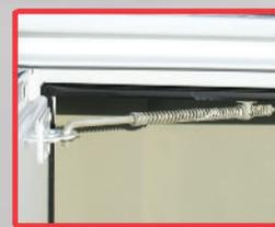
**G** Double spring over-center door retainer on all vertical doors eliminates involuntary swing and keeps the door in positive open or closed position.
