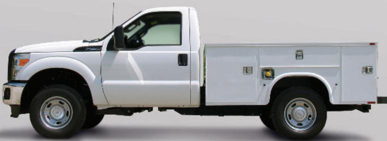
Low Profile Bodies offer greater visibility from the cab while only sacrificing 4" of body height compared to a standard service body.
