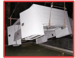
**N** Complete immersion in Knapheide's electro-deposition prime paint system for superior corrosion resistance.
