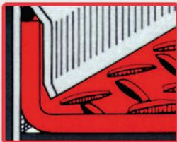
**B** Exclusive "Return Flange" floor design provides support for side compartments, adds floor strength, and eliminates rust-prone exposed seam between floor and side compartments.
