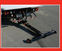
3. Optional Wheel Lifts/Tow Bars/Tow Hitches Wheel lifts and tow hitches include No-Lube™ pivot joints.
