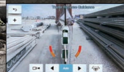
Trailer Reverse Guidance 1 automatically switches between side and rear camera views to show you what is most relevant while backing up your trailer, and provides overlays to guide you.
