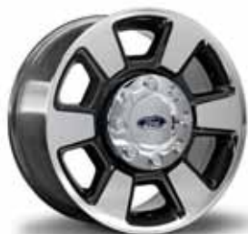
18" Bright-Machined Cast-Aluminum Standard on F-350 SRW
