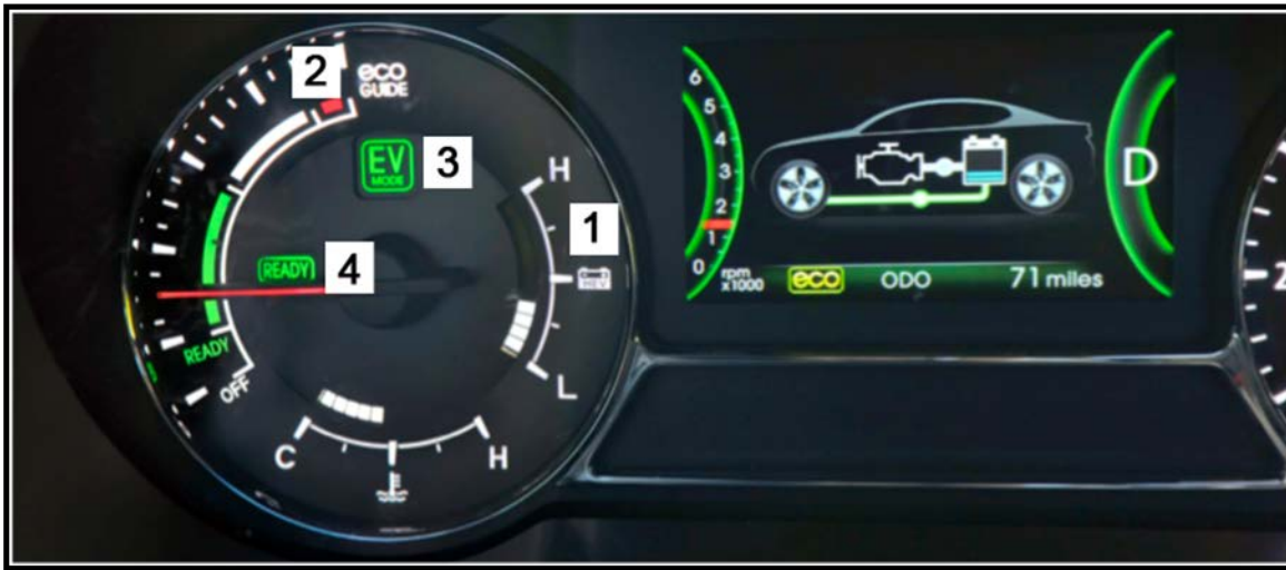
1. State of Charge(SOC) Gauge. 2. ECO Guide Gauge.3. EV Mode Indicator. 4. Ready Light.
