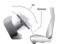
The foot-controlled release on the adjustable steering column lets both hands stay on the wheel while providing an infinite number of adjustments.
