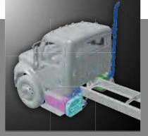
CLEAR BACK OF CAB TAILPIPE Clear left-hand and right-hand transmission PTO mounting locations
