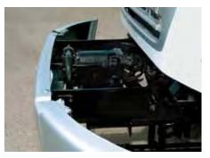
Integral front frame extensions on Business Class 106V and 112V models are designed to accommodate front-mounted PTOs and winches.
