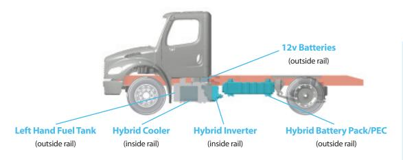
50 gallon left side fuel tank and under cab battery box shown. More fuel options available.
