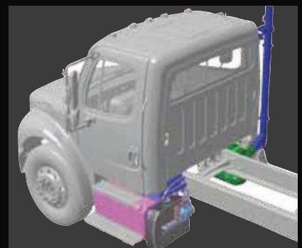
EPA 10 exhaust packaging provides the clear back of cab beverage body builders require, including alternate DEF pump locations.
