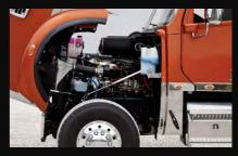
The hood tilts almost 90 degrees for easy engine access and serviceability.
