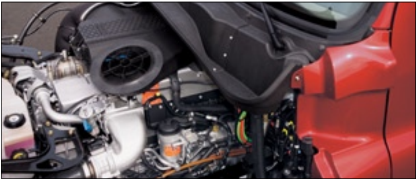
A detachable three-piece rain tray provides quick rear engine access. The removable middle section puts the top of the engine at your mechanic's fingertips.
