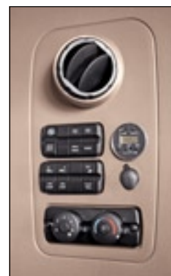
A wall-mounted console controls all of the sleeper conveniences, including HVAC and the dome light.
