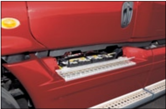
Batteries are accessed through a door and latch system built into optional side fairings.
