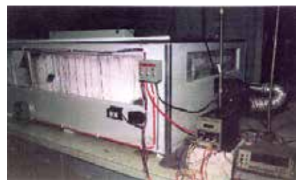
Corrosion chamber simulates prolonged exposure to the harshest environments.
