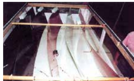
Protected sheet metal test panels and unprotected control panels are scribed and exposed to 800 hours of humidity @ 95°F.
