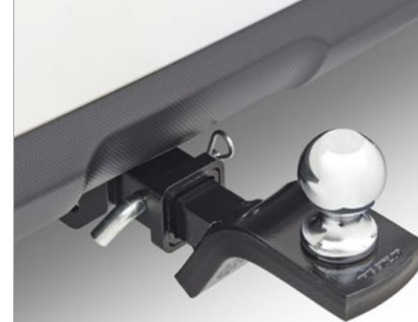
■ Trailer Hitch Subaru hitches are engineered to the same rigorous standards as the rest of your Outback. The hitch is rated at 3,000 lbs. maximum towing capacity with 3.6L engine (2,700 lbs. maximum with 2.5L engine) and 200 lbs. maximum tongue weight. L101SAL011 Hitch ball not included. Trailer brakes may be needed. Not compatible with Rear Bumper Underguard.
