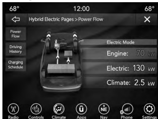
Power Flow Screen
