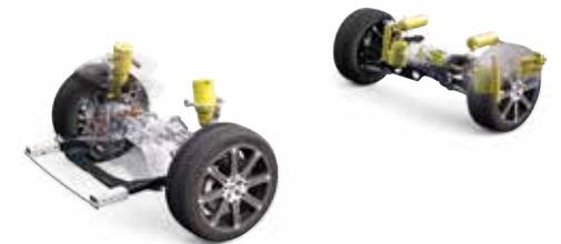
Air suspension on all four wheels gives the XC60 outstanding ride comfort – the air springs absorb imperfections in the road – and make the car stable by keeping the ride height constant, regardless of the load. With the active chassis you can alter the way the car rides and handles to suit your mood or the road.
