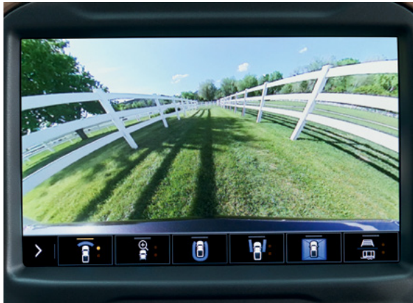
Front Camera View Displays front view with available guidelines to assist with parking and tight manoeuvres.
