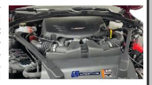
Finally, we have to mention the fourth-place 5.5L V8 LT6, the highest-ranked naturally aspirated engine on our list. Equipped by the C8 Chevy Corvette Z06, the high-revving LT6 is rated at 670 horsepower at 8,400 rpm and 460 pound-feet of torque at 6,300 rpm, making for 122.6 horsepower per liter.
