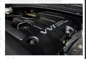
In second place in our list, we have the twinturbocharged 3.6L V6 LF4, currently equipped by the Cadillac CT4-V Blackwing and rated at 472 horsepower at 5,750 rpm and 445 poundfeet of torque 3,500 rpm, making for 132.4 horsepower per liter. To note, the LF4 was previously available for the now-discontinued Cadillac ATS-V, where it made 464 horsepower and 445 pound-feet of torque.
