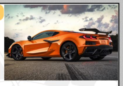
along with stickier Michelin Sport Cup 2 R ZP rubber, FE7 suspension with specially tuned Magnetic Ride Control 4.0 dampers, and available carbon fiber wheels that deliver a 41-pound reduction in unsprung mass. All Z07-equipped models also receive a full carbon fiber aerodynamics package with a larger front splitter, front-corner dive planes, a rear wing and an underbody strake. The aero kit produces 734 pounds of downforce at 186 mph.
