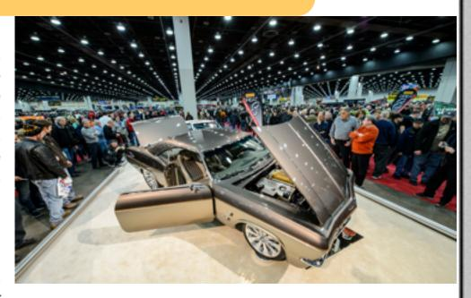
has been chopped, lowered, shortened, narrowed, and has an altered wheelbase. It was built for Canadian construction magnate Don Voth and contains a Corvette C6 drivetrain and suspension. Lastly, it holds the nickname Impostor.
