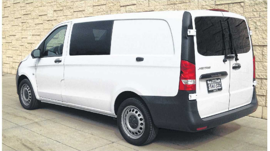
As a cargo van, Metris has up to 5.27 cubic metres of volume, up to 1,135 kilograms of payload and a side door wide enough to take a pallet. The bed is 283.1 cm (111.5 inches, or 9.3 feet) long by 168.5 cm (66.3 in. (5.5 feet)) wide. TODD GILLIS
