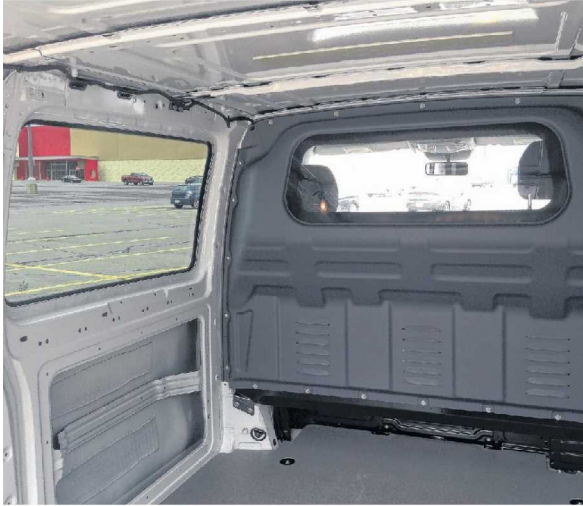
As a cargo van, Metris has up to 5.27 cubic metres of volume, up to 1,135 kilograms of payload and a side door wide enough to take a pallet. The bed is 283.1 cm (111.5 inches, or 9.3 feet) long by 168.5 cm (66.3 in. (5.5 feet)) wide. TODD GILLIS
