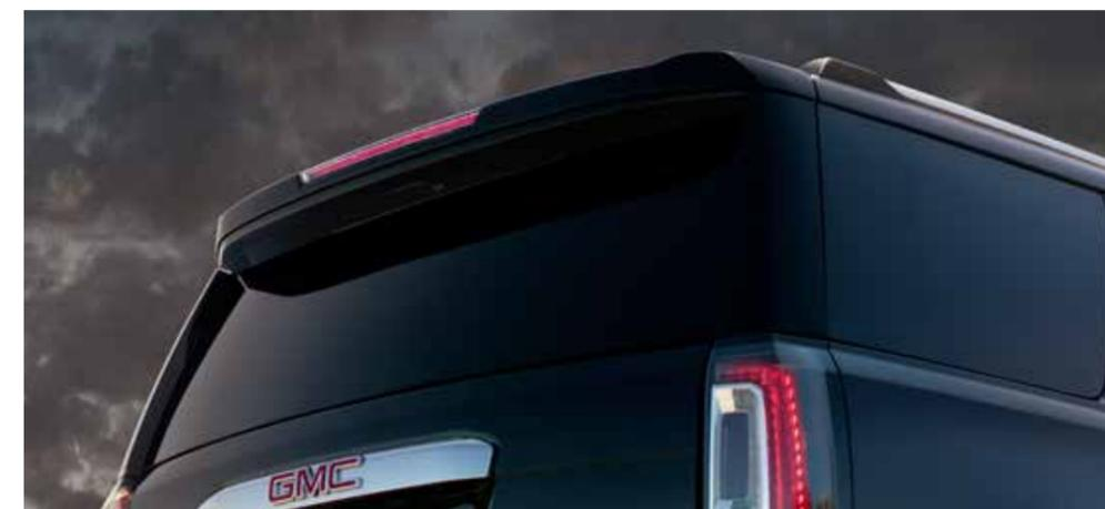
**REAR SPOILER** Located on top of the liftgate, the new spoiler houses a repositioned window wiper that is hidden when not in use for a clean, uncluttered appearance.
