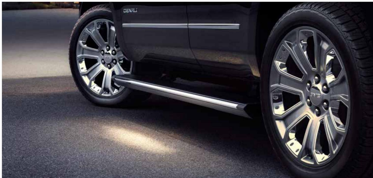
**POWER-RETRACTABLE ASSIST STEPS WITH PERIMETER LIGHTING** Yukon Denali models offer illuminated power-retractable assist steps that automatically extend when the front- or second-row doors are opened to provide easy, lighted access. They retract when the doors close for an uncluttered profile.
