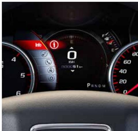
**CUSTOMIZABLE DRIVER DISPLAY** Choose Yukon Denali, and a reconfigurable gauge cluster allows you to personalize the new 203 mm (8") diagonal colour Customizable Driver Display for optimized information placement. The display's menu can be navigated with steering-wheel-mounted controls. Driver alerts are also clearly displayed.
