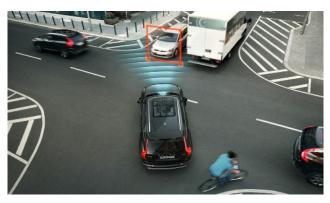
If a collision is imminent, at speeds above 10km/h, the front safety belts are tightened (option in 60 Series) to secure the driver's and front seat passengers' position.
