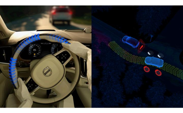
This system (standard in the 60 Series cars) helps the driver take evasive action in an emergency situation. If the driver faces a vehicle, cyclist, pedestrian, or a large animal in front, braking is not always enough – steering away is sometimes necessary to avoid an accident.
