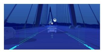
The driver can override the system at any time by using the brake pedal, accelerator pedal or steering wheel. Using the turn indicator will temporarily abort the steering support if the driver wants to change lane.
