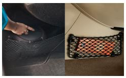
**Net Pocket Kit** A kit with three mesh pockets, two for the side panels in the cargo compartment and one for the tunnel console in the passenger compartment.
